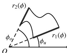
$$F = \frac{1}{2} \int_{\phi_u}^{\phi_o} (r_1^2 - r_2^2) \partial\phi \quad (119)$$
