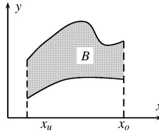
$$I = \int_{x=x_u}^{x_o} \left( \int_{y=h(x)}^{g(x)} f(x, y) dy \right) dx \quad (228)$$
