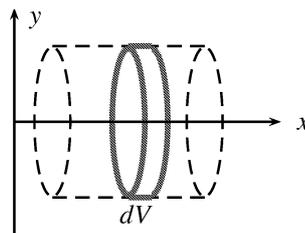
$$dV = Q \cdot dx \quad \Rightarrow \quad V = \int_a^b Q(x) dx \quad (95)$$
